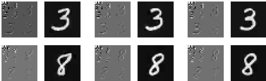
Figure 16: Digits generated with \text{Top-}p = 0.6 along with a depiction of the generated wavelet coefficients.
